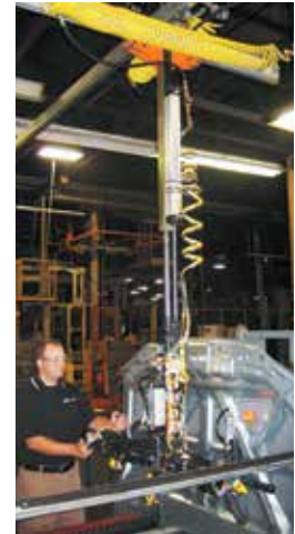
Torque tube with integrated vacuum handling device
